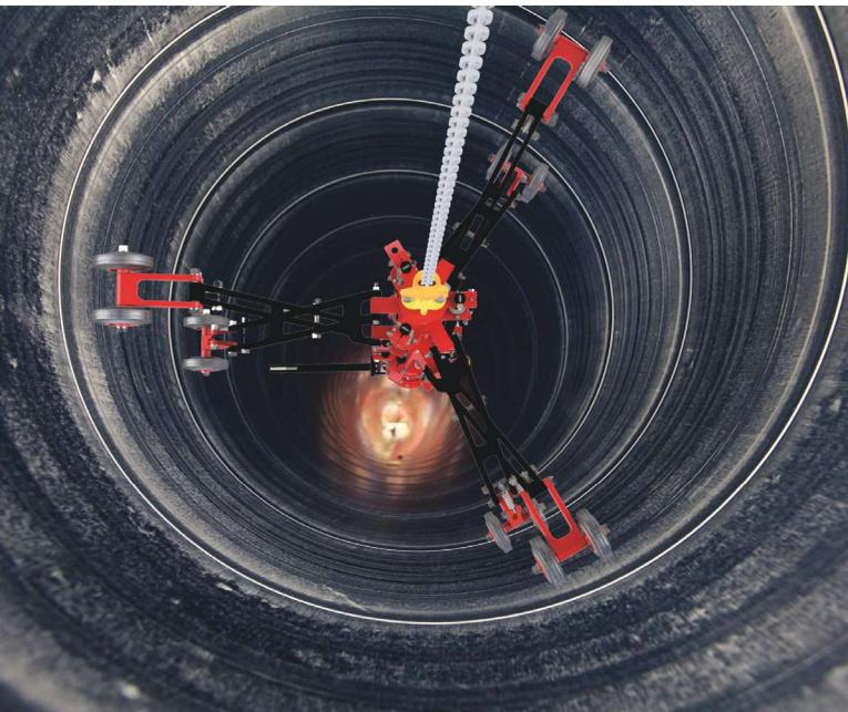
The SIRIUS-X is shown performing a caisson inspection. (Source: AISUS)
